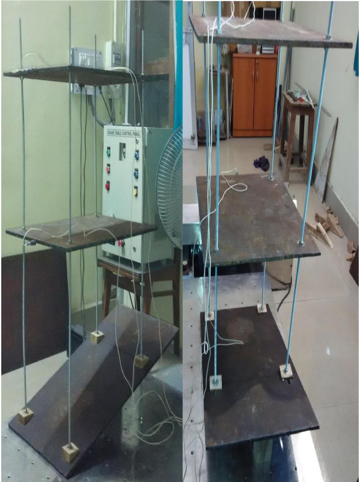
Figure 3.7: Experimental Model for 20° slope
